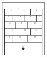
Narrow down the width on the first row or as a minimum cut off the tongue to achieve the first distance to the wall. If the wall is curved or uneven the first row has to be cut and copy the contour of the wall. Use spacers! Cut off the tongue on the first plank also on the short side. This plank will then have the plastic tongue in the end to the right.
